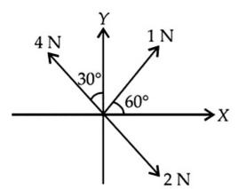
Three forces acting on a body are shown in the figure. To have the resultant force only along the y -direction, the magnitude of the minimum additional force needed is (2008)
