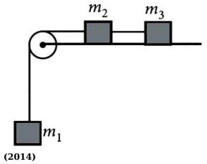
A system consists of three masses  $m_1$ ,  $m_2$  and  $m_3$  connected by a string passing over a pulley P. The mass  $m_1$  hangs freely and  $m_2$  and  $m_3$  are on a rough horizontal table (the coefficient of friction =  $\mu$ ). The pulley is frictionless ad of negligible mass. The downward acceleration of mass  $m_1$  is
