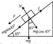
The various forces acting on the body have been shown in the figure. The force on the body down the inclined plane in presence of friction  $\mu$  is  $F = mg \sin \theta - f = mg \sin \theta - \mu N = ma$
