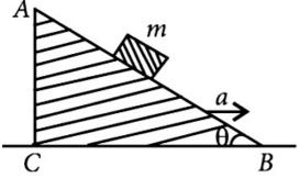
The wedge is given an acceleration a towards the right. The relation between a and  $\theta$  for the block to remain stationary on the wedge is (NEET 2018)
